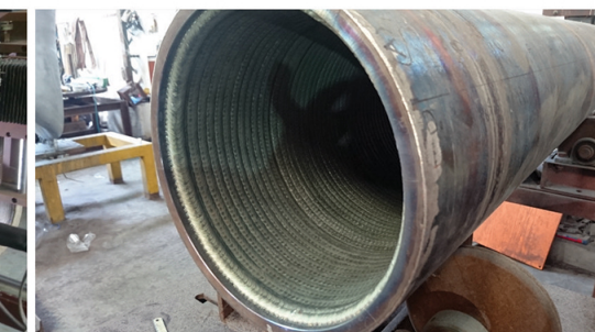
Cladded Pipe 2Meter Long
