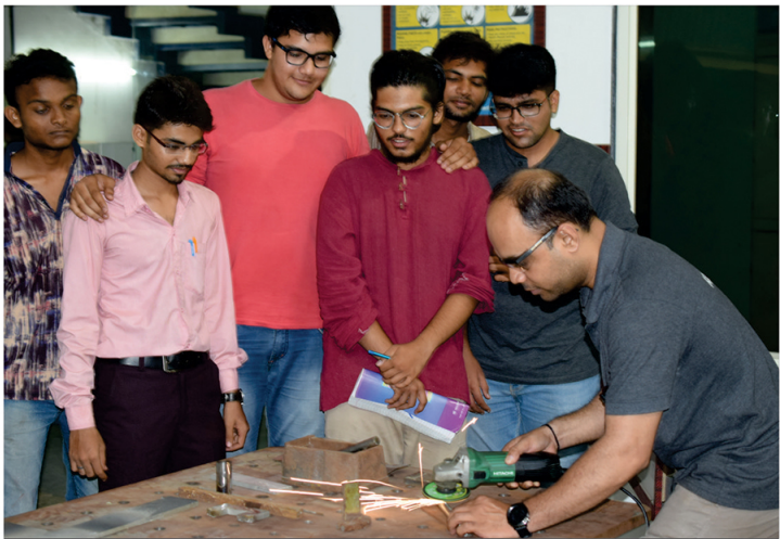
Identification of Material with Spark Test
