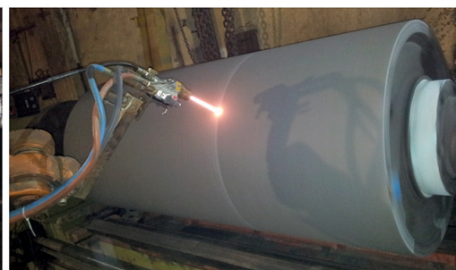
HVOF Process Tungsten carbide on Bridal Roll
